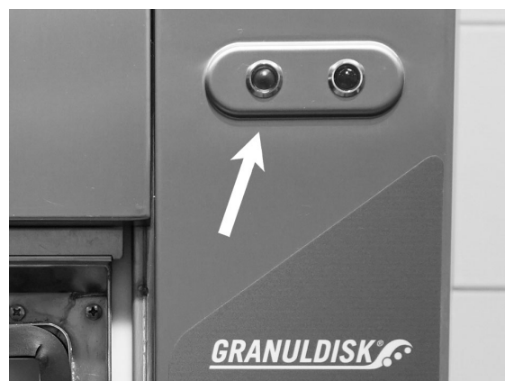
Fig. 23 When the program is finished the green light goes on.
