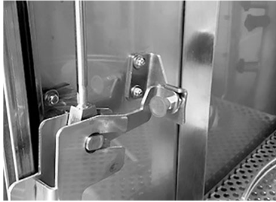
Fig. 28 Close up – secure the arm properly
